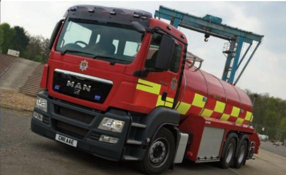
of the critical specification factors, during this bidding process. He explains that his team has already worked hard ensuring that its new vehicles are as light and fuel-efficient as possible, to the point where everything now fits on a 12-tonne chassis. “So we were also keen to reduce vehicle height, because, with ageing fire stations, we haven’t got space to get a heavier or taller chassis in,” he says.
